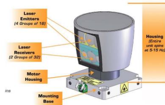
Figure 3.21. General architecture of laser scanners (Source: Velodyne)
