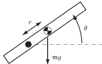
$$\begin{aligned}\tau &= M\ddot{\theta} + mgr \cos \theta + b\dot{\theta} \\ &= M\ddot{\theta} + h(\theta, \dot{\theta})\end{aligned}$$
