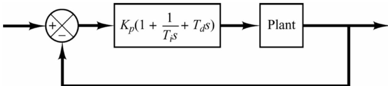
$$\frac{U(s)}{E(s)} = G_{PID}(s) = K_P + K_I \frac{1}{s} + K_D s = K_P \left( 1 + \frac{1}{T_I s} + T_D s \right)$$
