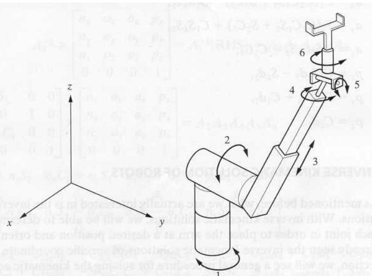
**Figure 2.29** Schematic drawing of the Stanford Arm.
